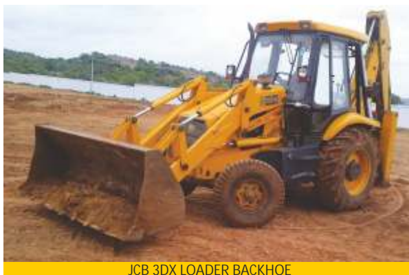
JCB 3DX LOADER BACKHOE
